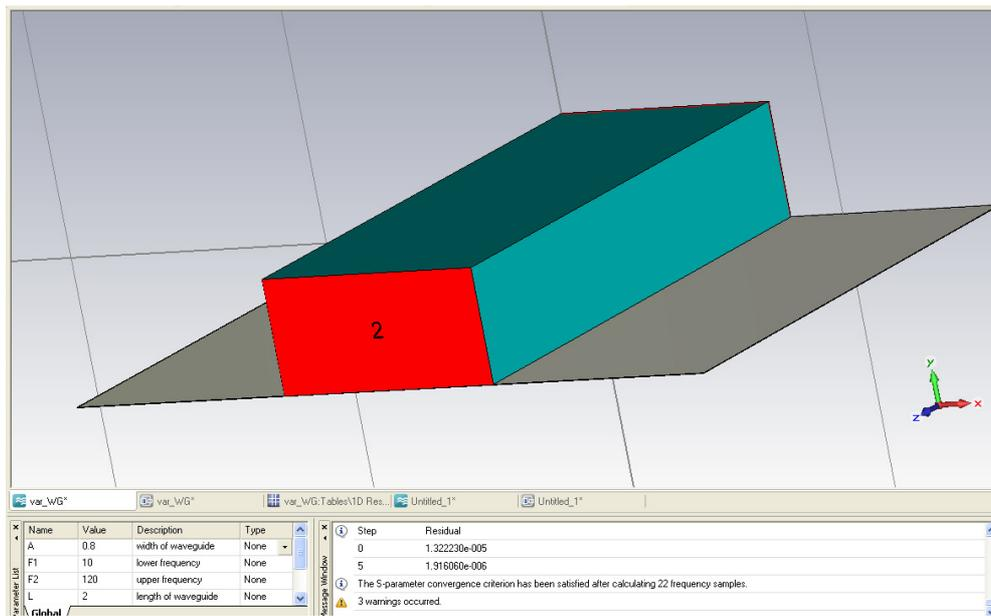
Figure 4: WR-2.5 Dielectric Image Waveguide
