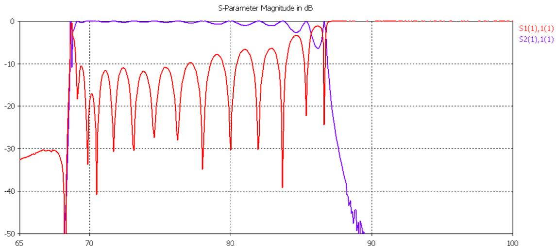
Figure 9: Dielectric-waveguide filter response with no. of gating = 16
