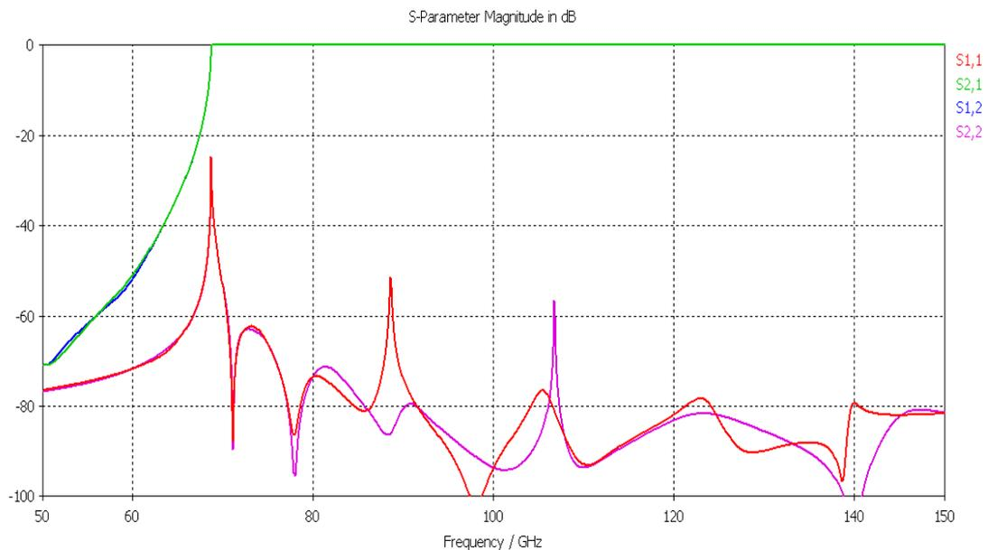
Figure 7: s-parameter of dielectric waveguide WR-2.5
