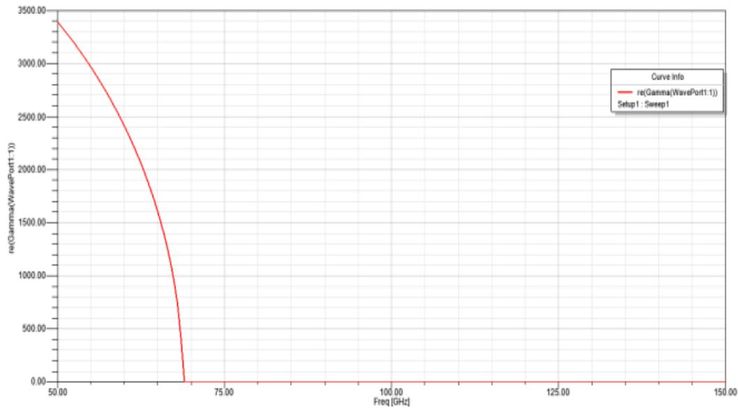
Figure 6: attenuation constant of dielectric waveguide WR-2.5
