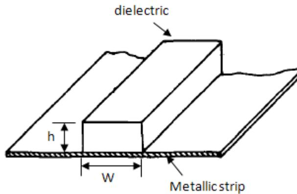
Figure 1: Typical micromachined Dielectric waveguide
