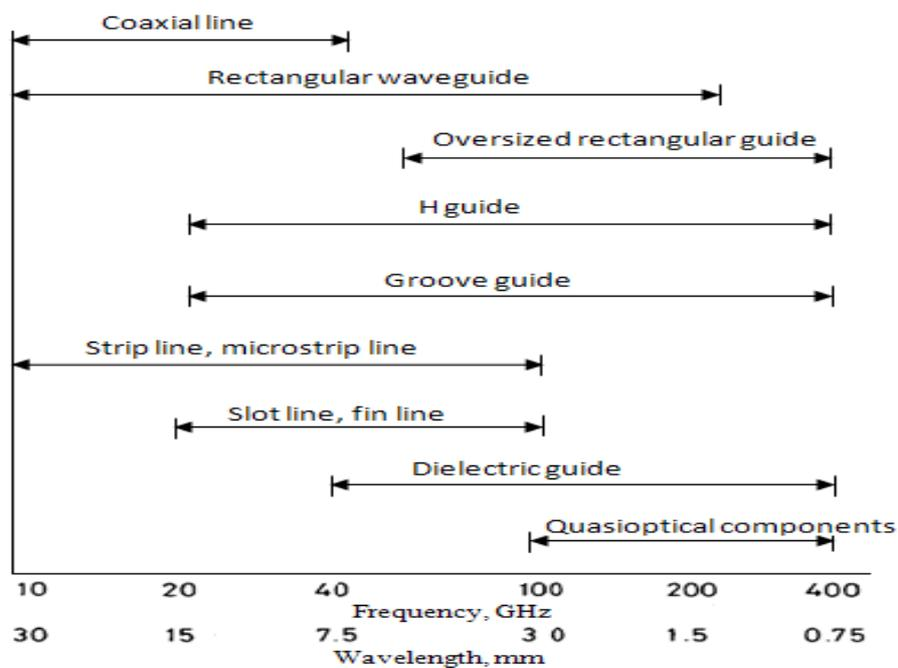
Figure 2: Useful ranges of millimeter waveguide
