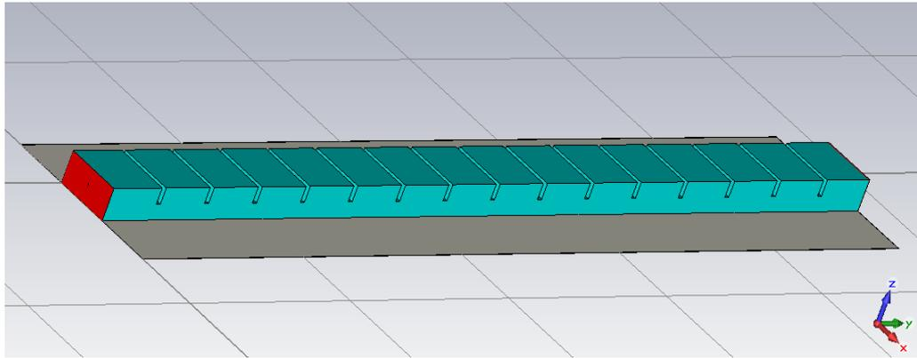
Figure 8: the dielectric-waveguide (DW) with upper notches filter with no. of gating = 16
