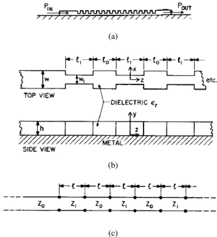
**Figure 3** the dielectric-waveguide (DW) (a) with upper notches (b) with side notches (c) An equal-line-length equivalent circuit for gratings [3]
