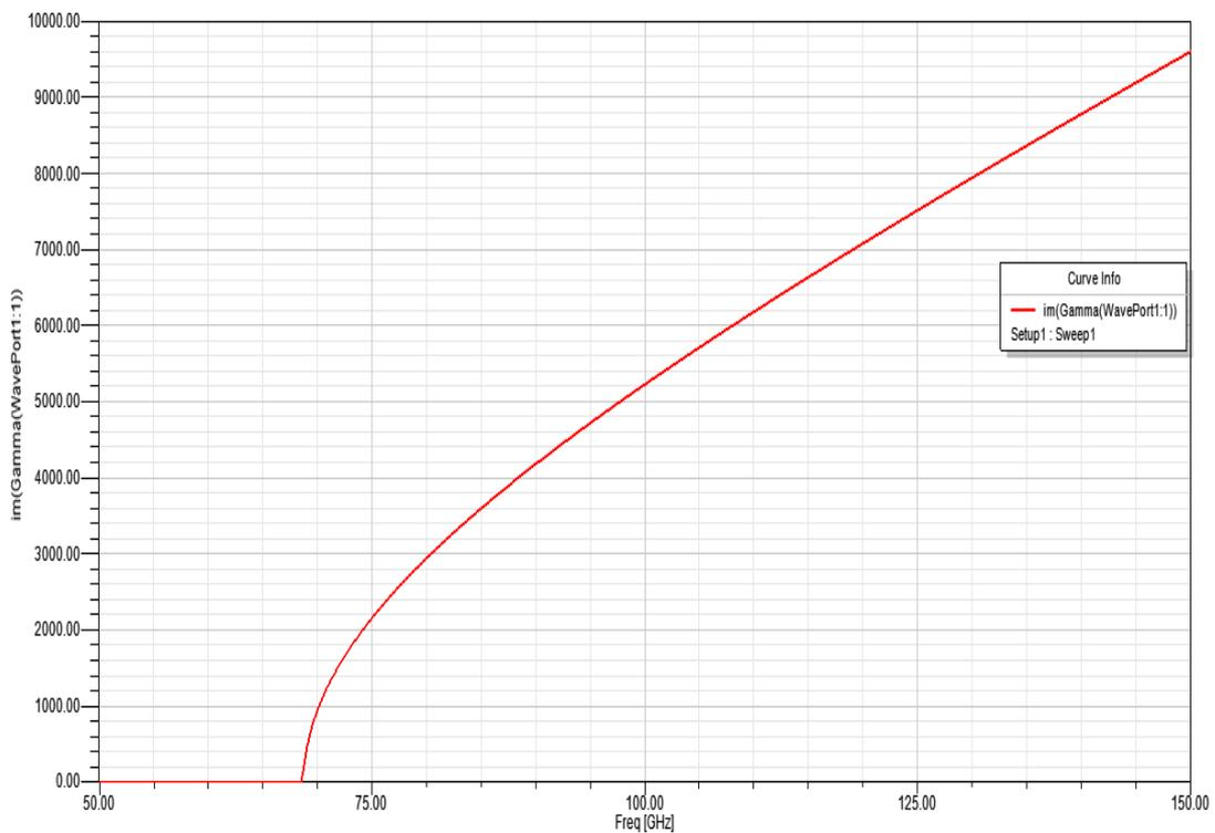
Figure 5: propagation constant of dielectric waveguide WR-2.5
