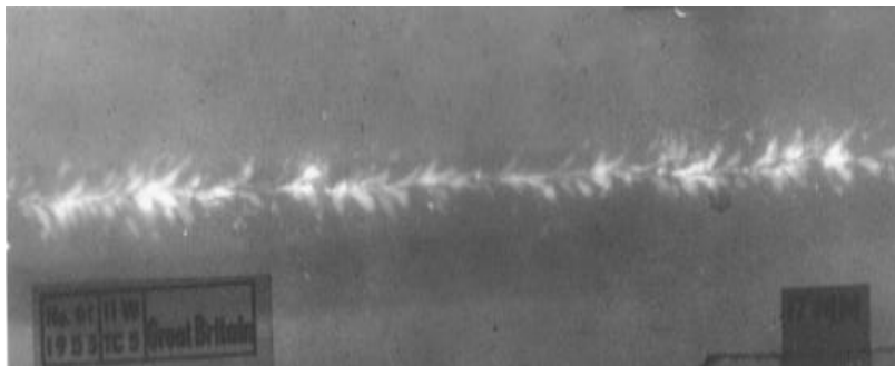
Fig. 6 Original X-Ray image having Gas- cavity (worm hole) type flaws
