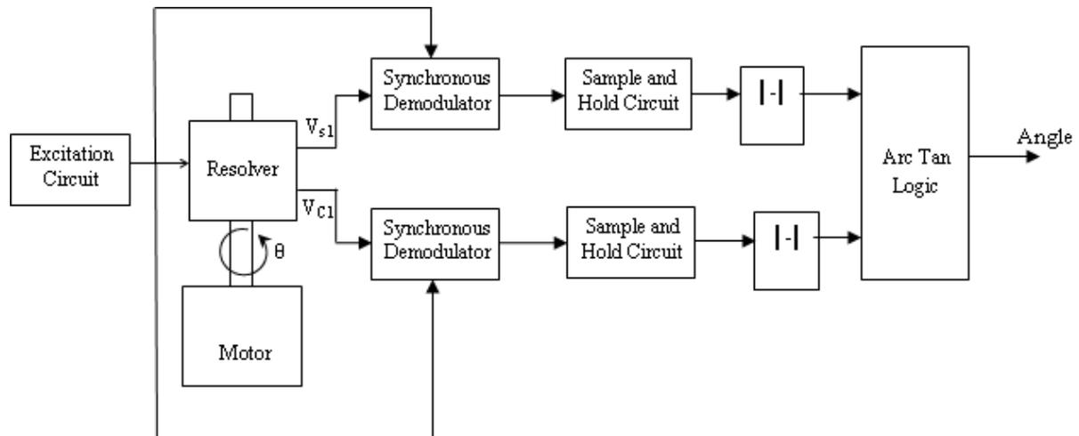
Figure 4. Block diagram of proposed RDC using inverse tangent method
