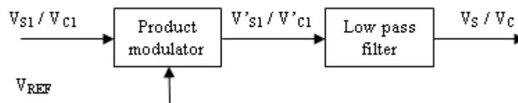
Figure 5. Synchronous demodulator
