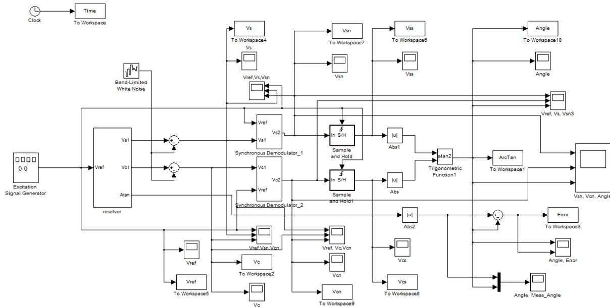
Figure 7. MATLAB® Simulink model of RDC using inverse tangent method
