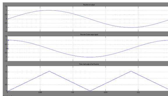
Figure 14. Demodulated resolver output signals
