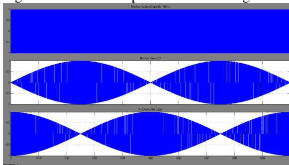
Figure 9. Resolver excitation and output signals (600rpm)
