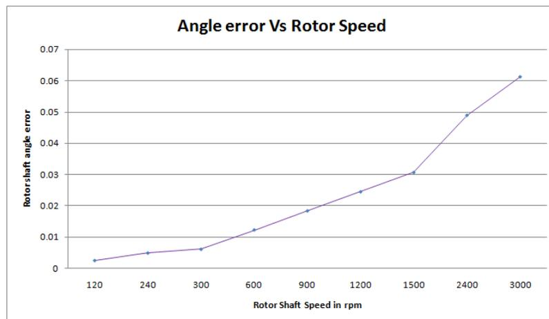
Figure 17. Graph between rotor shaft angle error and rotor speed
