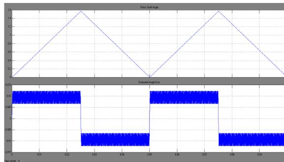
Figure 12. Measured angle and rotor angle error
