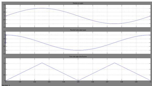
Figure 11. Resolver demodulated output signals and angle
