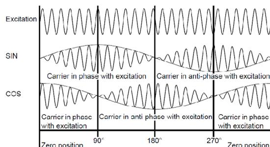
Figure 3. Resolver excitation and output signals
