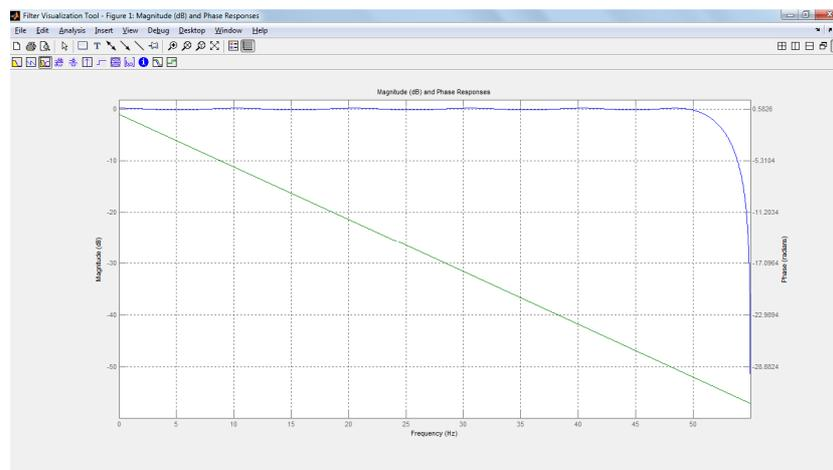
Figure 8. Frequency response of the low pass filter
