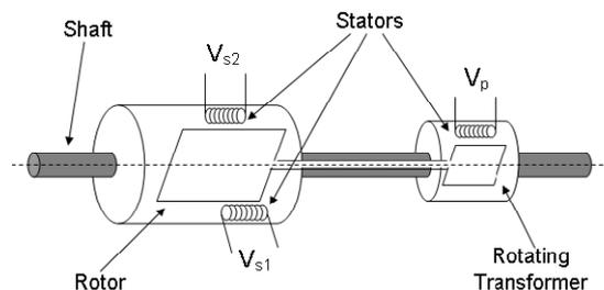
Figure 1. Internal view of a resolver
