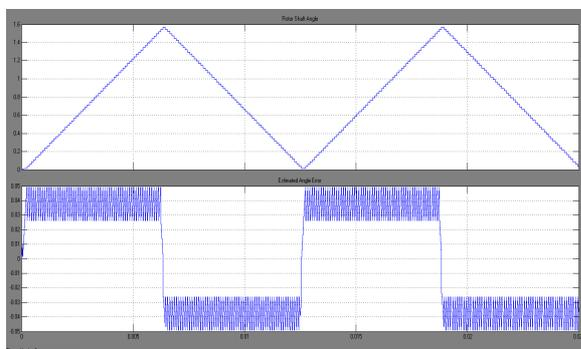
Figure 15. Measured angle and rotor angle error
