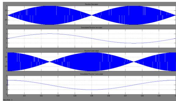
Figure 10. Demodulated resolver output signals
