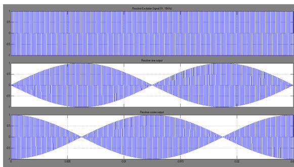
Figure 13. Resolver excitation and output signals (2400rpm)
