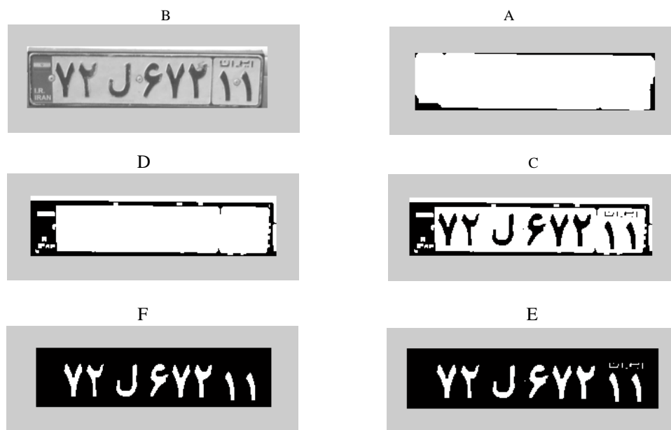
Fig.8. Character detection, (a) selected object with plate binding box,(b) extracted plate from fig.7.a, (c) Thresholded plate, (d) filled plate, (e) result of XOR between c and d, (f) after removing the available noise
