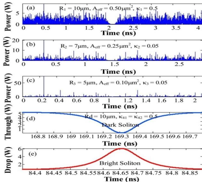
Fig. 3: Results of the soliton signal within the ring resonator system, where (a)  $R_1$ , (b)  $R_2$ , (c)  $R_3$ , and (d) – (e) dark – bright soliton conversion at the add/drop filter.
