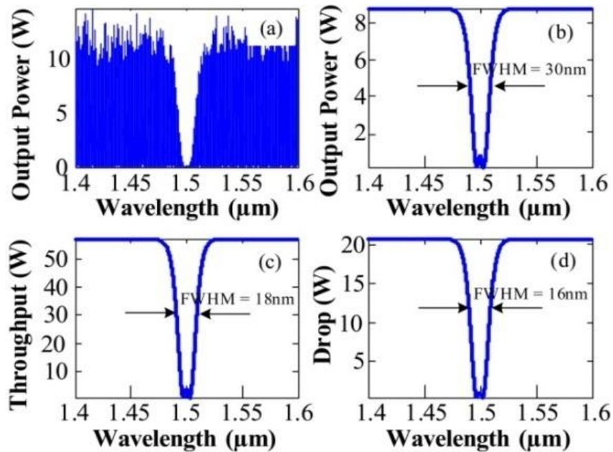
Fig. 5: Tuned dynamic optical tweezers output within an add/drop filter.
