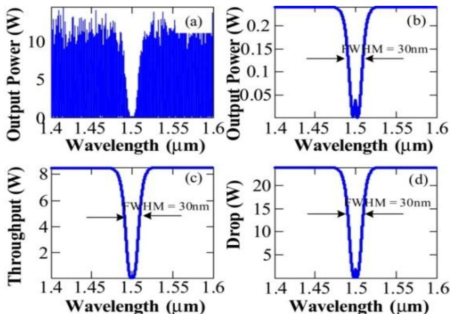
Fig. 4: The dynamic optical tweezers output within an add/drop filter, when the bright soliton input with the central wavelength  $\lambda_0 = 1.5\mu\text{m}$ .
