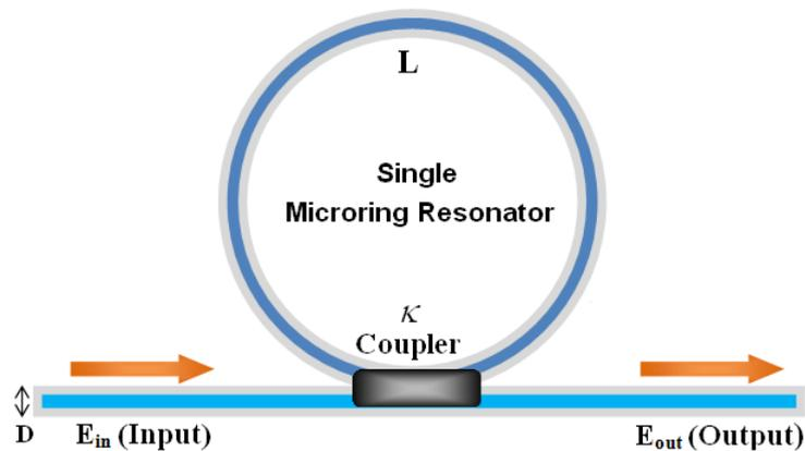
Fig.1: Schematic of nonlinear silicon MRR
