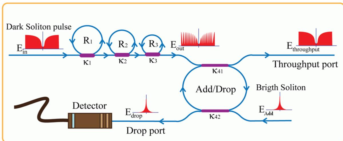
Fig. 2: Schematic diagram of a dark-bright soliton conversion system.
