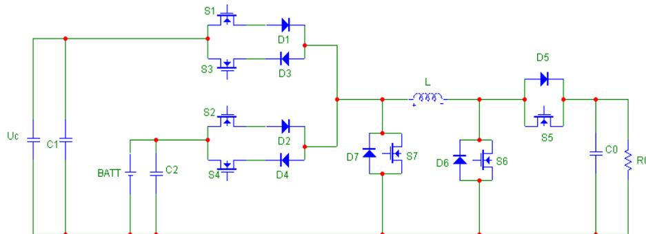
Figure 2. Multi-input power converter
