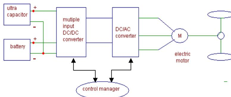
Figure 1.Proposed Block diagram of hybrid vehicle
