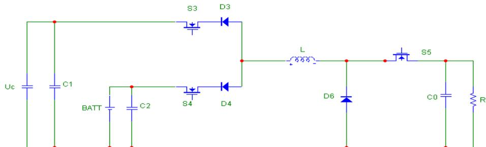
Figure 4. Buck mode converter
