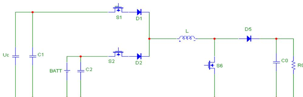
Figure 3. Boost mode converter
