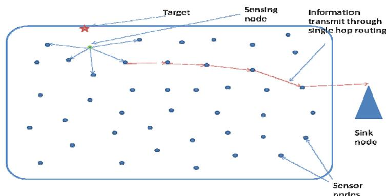
Figure 1. Target tracking using HCTA and single hop routing scenario.
