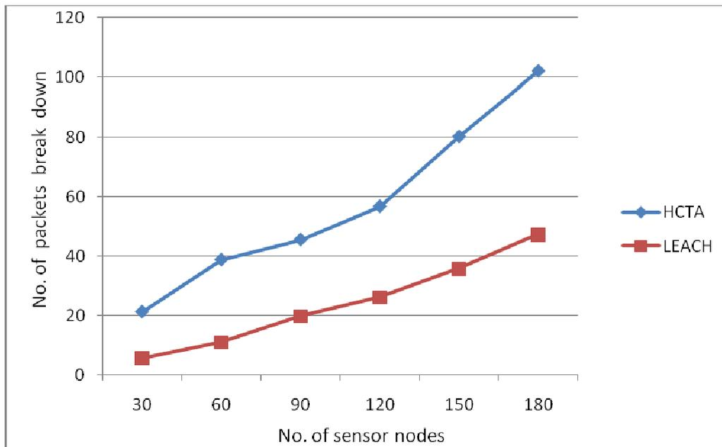
Figure 6. Number of packets breakdown at receiver
