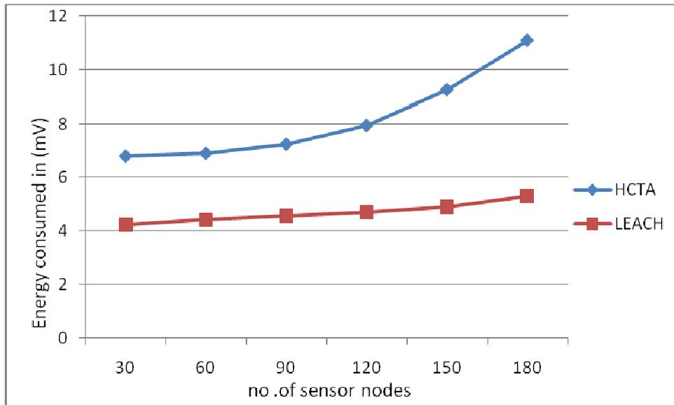
Figure 4. Energy consumed by sensor node
