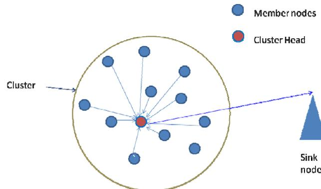
Figure 3. Each cluster have a CH and information receive from member nodes
