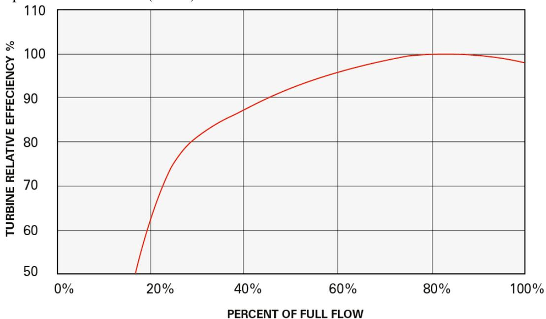
Fig. 5 Turbine Efficiency with full flow
