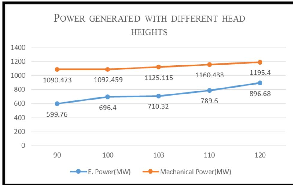
Fig 4: Power generated with different head height
