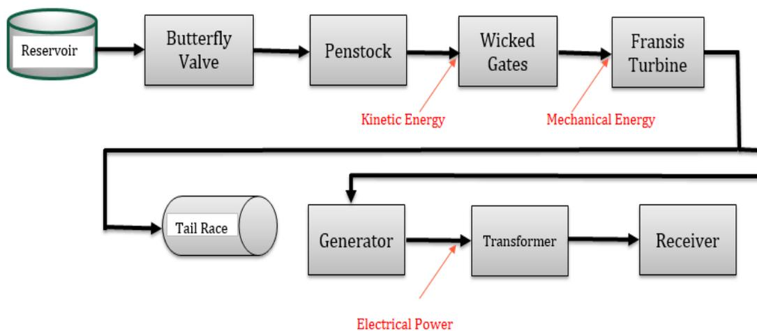
Fig 2. Schematic View of a Hydro Power Plant.
