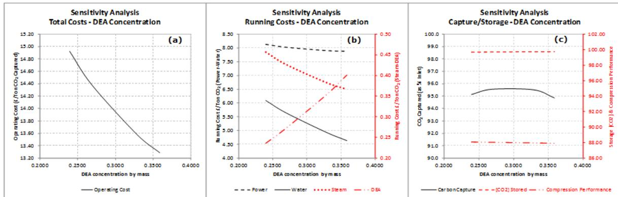
Figure 5: Sensitivity analysis of the CCS plant with respect to the DEA concentration used for absorption
